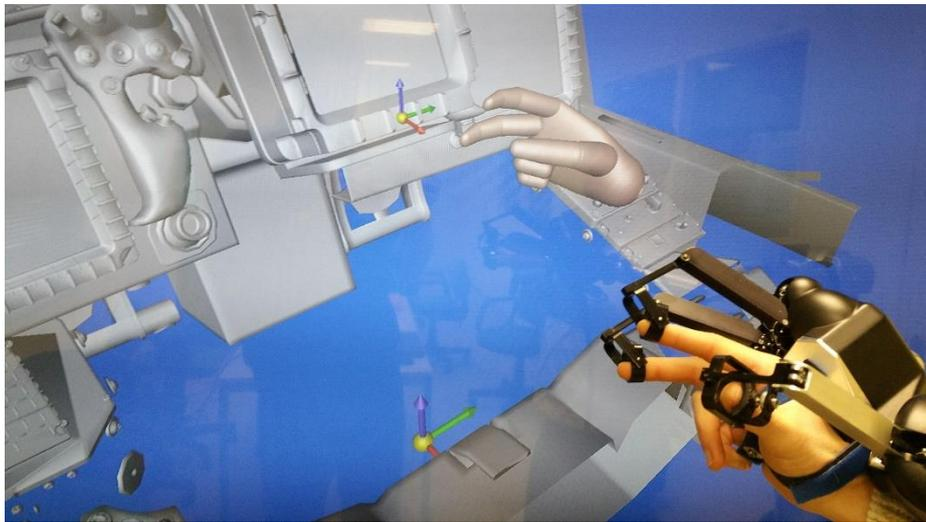
**Figure 1.** Prototype of the HGlove.
