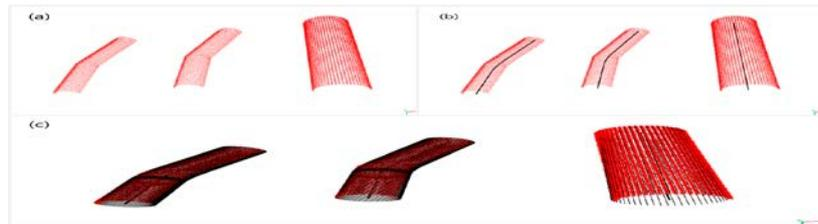
**Figure 1.** The result of multiple cylindrical objects detection. (a) is a synthetic point cloud, (b) is a result of axis modeling and (c) is a result of reconstruction. The number of points is about 44k.
